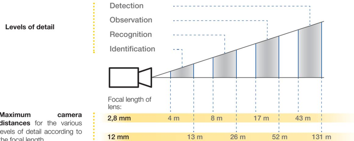
**Maximum camera distances** for the various levels of detail according to the focal length
